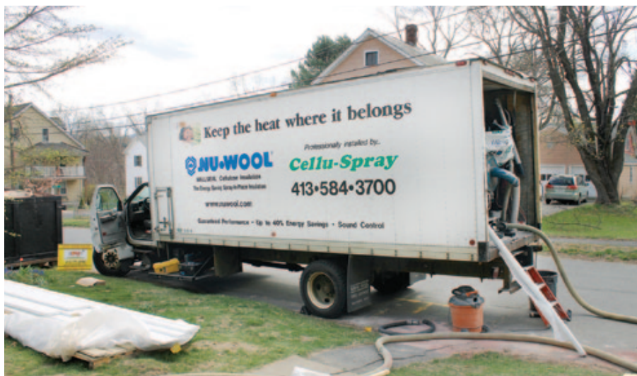
Figure 1. This truck (above) is equipped to install either damp-spray or dense-pack cellulose. The hopper that feeds material to the operator can be filled to the ceiling (right), providing enough material to last from 15 minutes to an hour, depending on the application.
